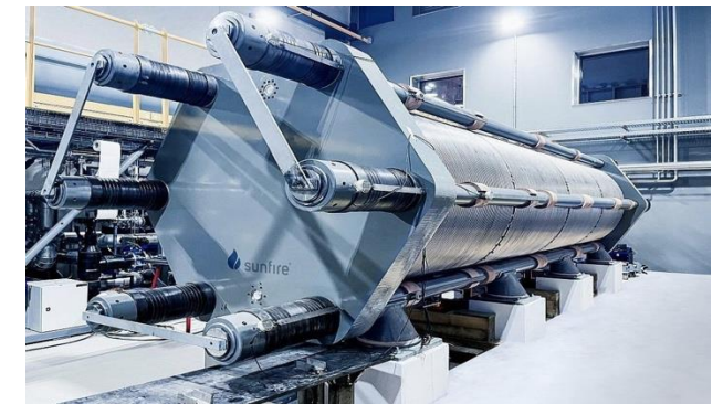
Sunfire 10MW alkaline electrolyser stack
