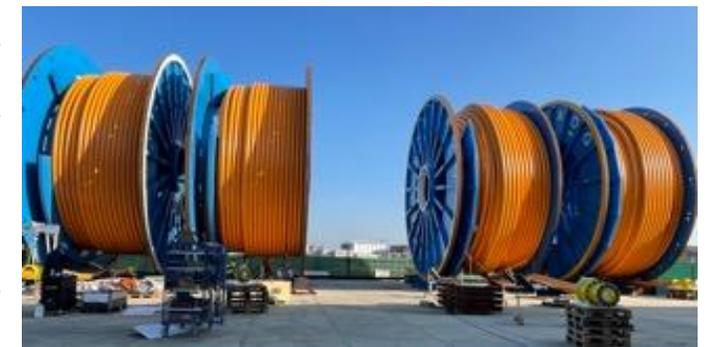
Strohm's TCP ready for installation offshore
