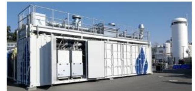
*Sunfire’s solid oxide cell electrolyzer*
